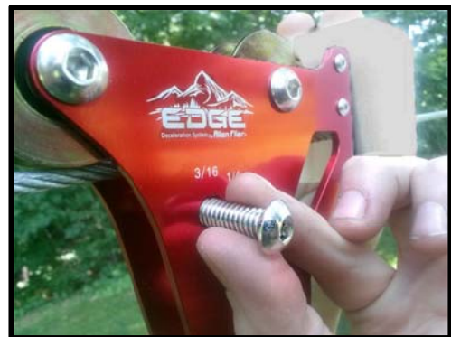
Insert the screw into the appropriate hole for your cable size, and the nylon washer between the red frames.
