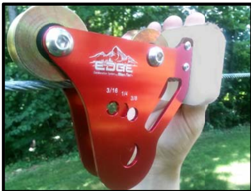
Put the unit onto your zip line, with the white bumper facing the upper tree.
