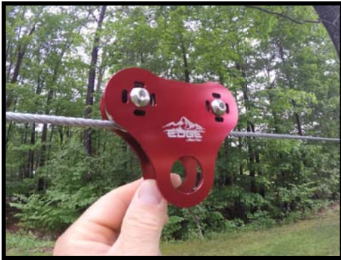
Drop the trolley onto the line.
