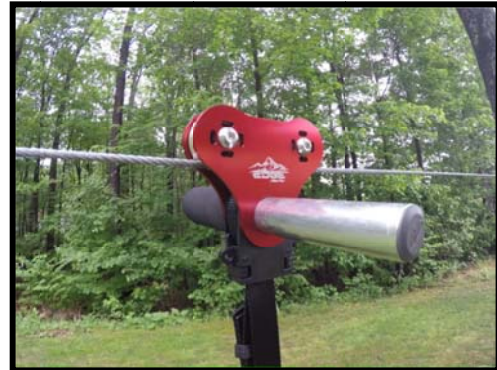
Press the spring button and push the handle in until it snaps firmly into the harness adaptor.
