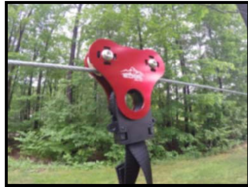
Align the large hole in the harness adaptor with the large hole in the trolley.
