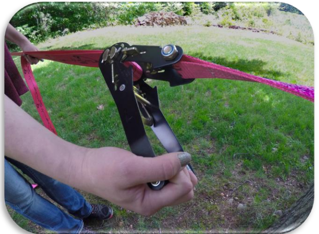
8. Using the ratchet, tighten the line to your desired tension.
