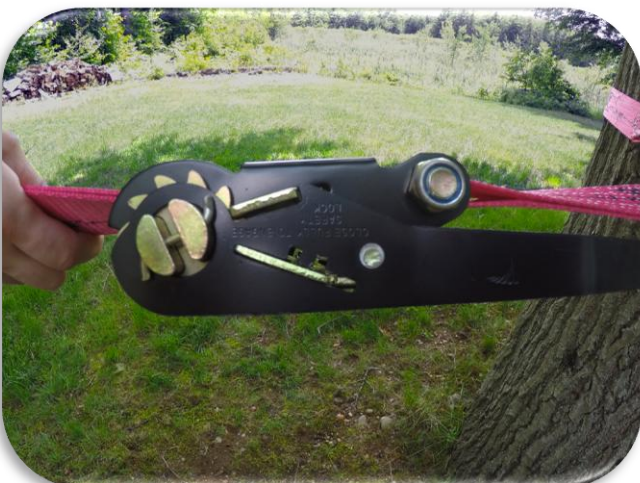
9. Close the ratchet, making sure it locks in place.
