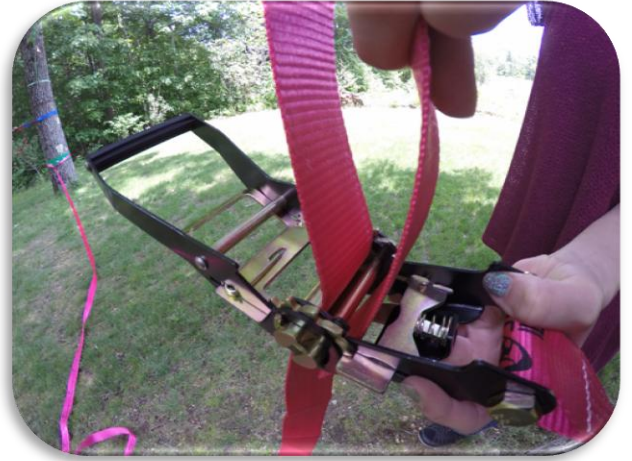
6. Open the ratchet and feed the line up and through the ratchet and back down.
