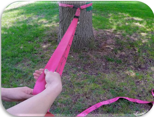
7. Pull the line through the ratchet.
